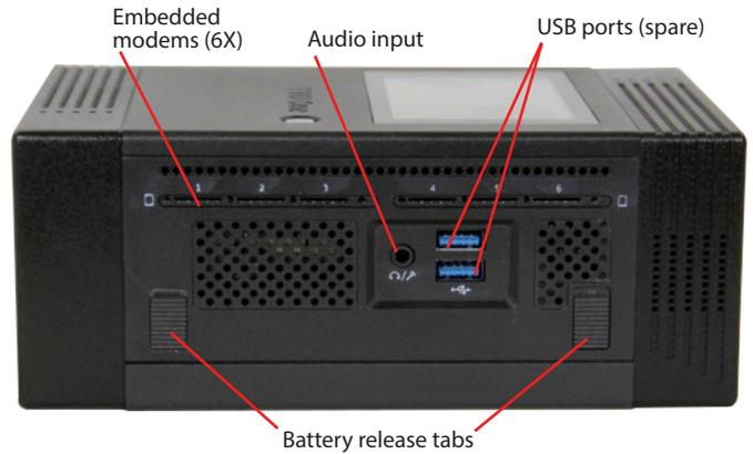
*TVU One model TM1000 v1 transmitter right-side panel*
