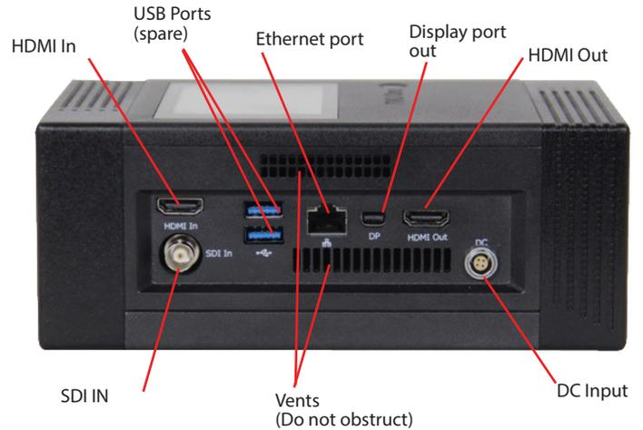
*TVU One model TM1000 v1 transmitter left-side panel*
