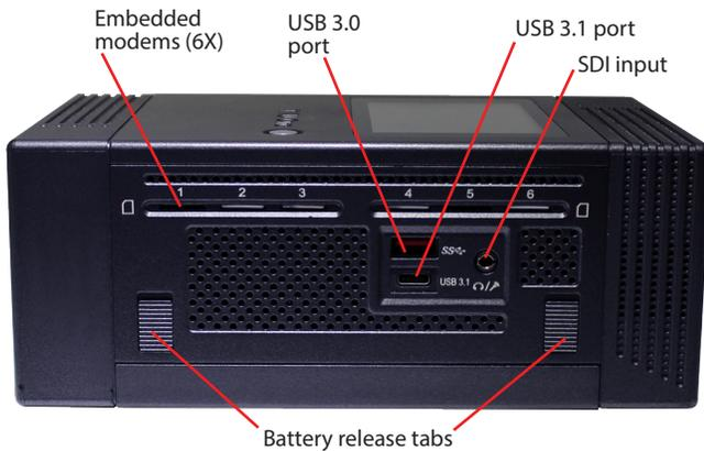
TVU One model TM1000 v2 transmitter right-side panel
